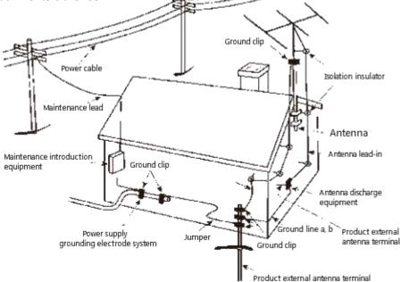
**Cable TV System Installation Instructions:** This instruction is used to alert the cable system installer to the National Electrical Code 820-40, which provides guidance on how to properly ground, especially when the ground wire is connected to the building grounding system. Near the wire lead-in point.
